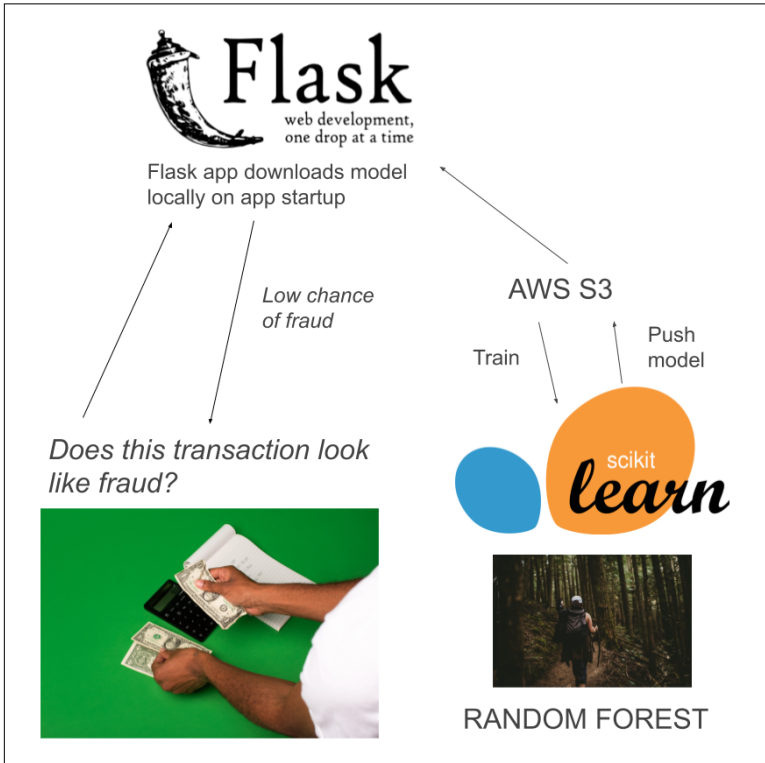
Figure 5-4. A Python Flask app can download models trained by a cron job so it can classify fraud
