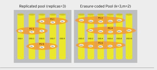
Figure 3. Graphical representation of relationships among Ceph storage pools, PGs, and OSDs, for both replicated pools and erasure-coded pools.
