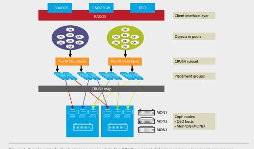
Figure 1. Clients write to Ceph storage pools while the CRUSH ruleset determines how placement groups are distributed across object storage daemons (OSDs).
