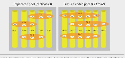
Figure 3. Graphical representation of relationships between Ceph storage pools, PGs, and OSDs, for replicated and erasure-coded pools.
