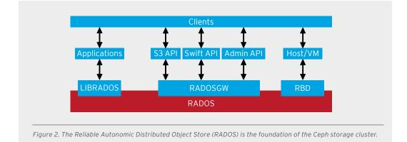
Writing and reading data in a Ceph storage cluster is accomplished using the Ceph client architecture. Ceph clients differ from competitive offerings in how they present data storage interfaces. A wide range of access methods are supported, including:
