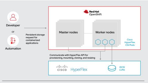
Figure 2: The Cisco HyperFlex CSI plugin for Red Hat OpenShift provides persistent storage for cloud-native workloads
