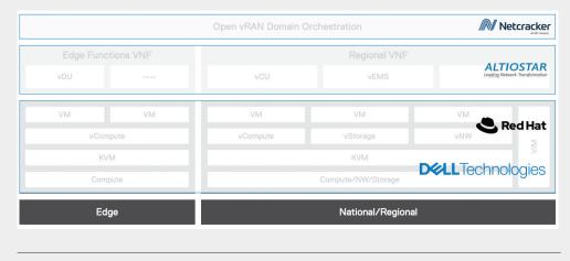
Figure 1: High-level reference architecture for vRAN
